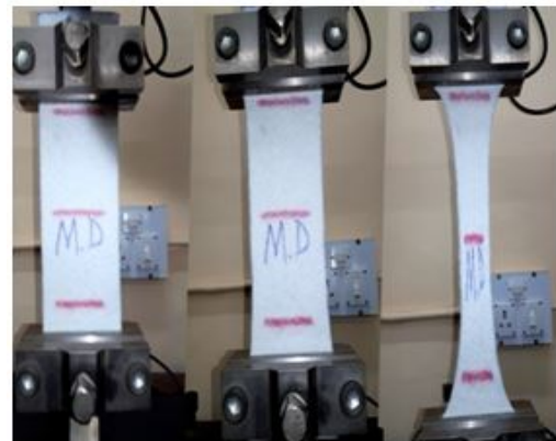
Figure 1. Distortion (waisting) of nonwoven fabric during tensile testing
